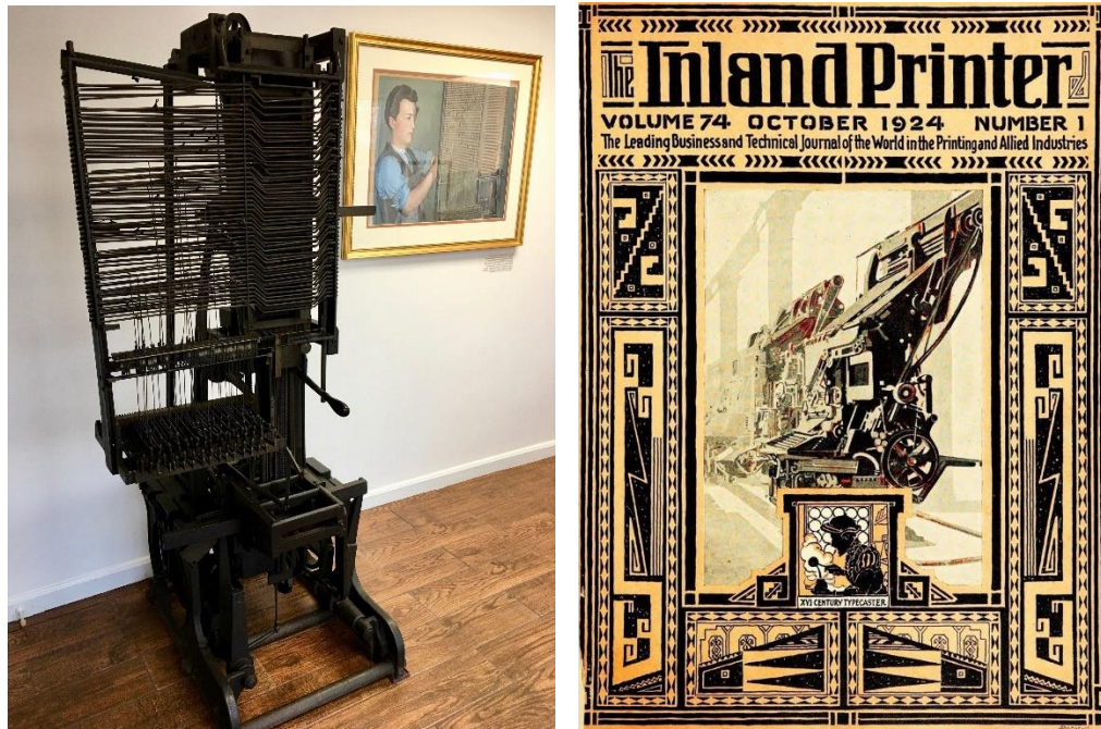
Figure 3: A Linotype Prototype Called the 1883 Second Band Machine (left); October 1924 Cover of The Inland Printer magazine (right)
